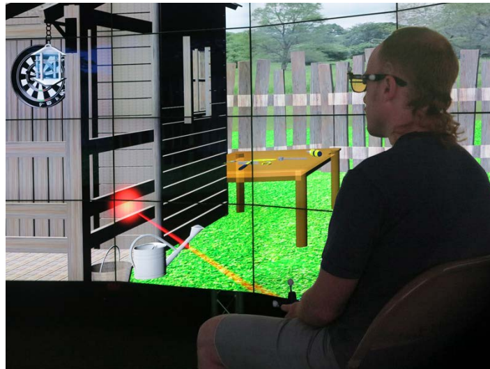
Fig. 5. Direct manipulation interaction in the CAVE2. By pushing a button on the Wand, the performer can point the virtual laser pointer and click on the watering can trigger object.
