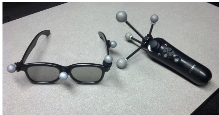
Fig. 2. CAVE2 input devices; the head and the wand controllers with retro-reflective markers for Vicon infrared optical tracking system.
